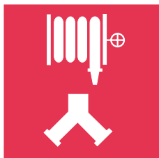
Fire Department Standpipe Connection
