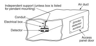
Figure A-2-10.5.2(b) Typical duct detector placement.
