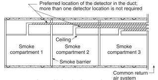
Acceptable location for a smoke detector in an air duct
