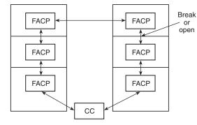
Style 7 fiber network where the panel has a two-way path communications capability, with one break. System remains as one LAN and meets Style 7.
