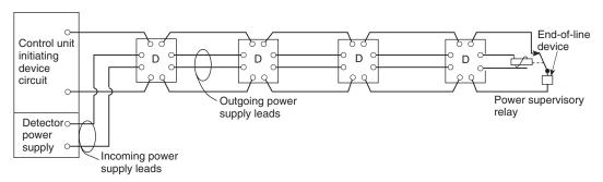
Illustrates four-wire smoke detector employing a four-wire connecting arrangement. Incoming and outgoing leads or terminals for both initiating device and power supply connections. Wire run broken at each connection to provide supervision.
