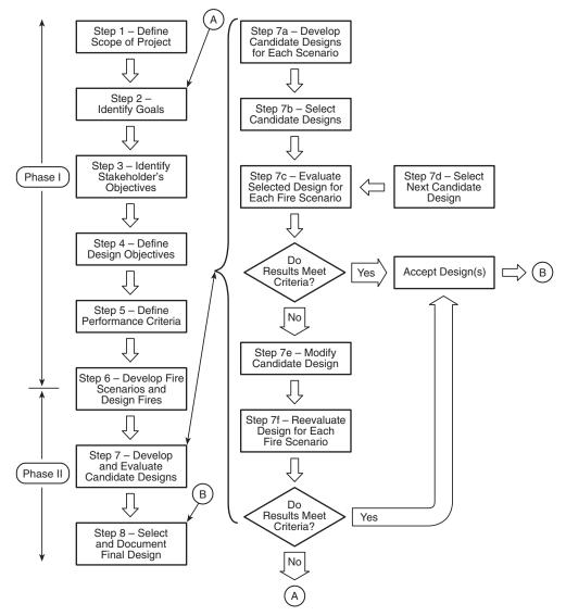
**B-2.2.1.1** While defining the project's scope, the designer will identify which of the three situations in Table B-2.2.1.1 best describes the project at hand (that is, a performance-based analysis of an existing detection system in an existing building).
