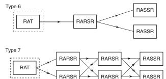
Figure A-7-2.2(b)(14)(e) One-way radio alarm system.
