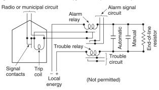
Figure A-6-16.4.1(b)(2) Shunt-type auxiliary fire alarm system.
