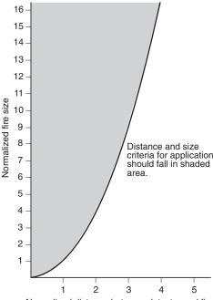
Figure A-2-4.3.1.1 Normalized fire size vs. distance.
