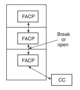
Style 4 fiber network where the panel has a two-way path communications capability. A single break separates the system into two LANs both with Style 4 capabilities.
