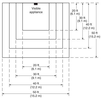
Note: Figure 4-4.4.1.1 is based on locating the visible signaling appliance at the halfway distance of the longest wall. In square rooms with appliances not centered or nonsquare rooms, the effective intensity (cd) from one visible signaling appliance shall be determined by maximum room size dimensions obtained either by measuring the distance to the farthest wall or by doubling the distance to the farthest adjacent wall, whichever is greater, as shown in Table 4-4.4.1.1(a).
