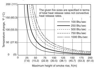
Figure B-4.1.2.3.8.7 Temperature change and maximum height of smoke rise for given fire sizes.
