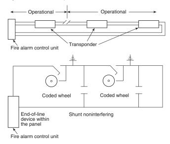
(11) *Style 5.0 (Class A)*. Verify the alarm receipt capability and trouble annunciation by lifting a conductor and actuating a multiplex interfacing device or a transmitter on each side of the break. For the earth ground verification, place an earth ground and certify alarm receipt capability and trouble annunciation by actuating a single multiplex interfacing device or a transmitter.
