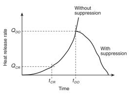
**B-2.3.2.2.1** Once the design objectives and the design fire have been established, the engineer will need to establish two points on the design fire curve:  $Q_{DO}$  and  $Q_{CR}$ .
