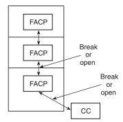
Style 4 fiber network where the panel has a two-way path communications capability. A double break isolates the panels and the control center in this case. In this case, there is one LAN and one isolated panel operating on its own. Control center is isolated completely with no communications with the network.
