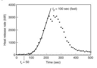
**B-2.3.2.1.2.9** For purposes of this appendix, fires are classified as being either slow-, medium-, or fast-developing from the time that established burning occurs until the fire reaches a heat release rate of 1000 Btu/sec (1055 kW). Table B-2.3.2.1.2.9 results from using the relationships discussed above. *[See also Table B-2.3.2.3.1(a).]*
