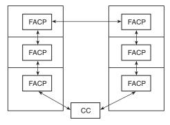
Style 7 fiber network where the panel has a two-way path communications capability.
