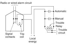
Figure A-6-16.4.1(a)(2) Local energy-type auxiliary fire alarm system.
