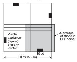
Figure A-4-4.1(d) Room spacing allocation — incorrect.
