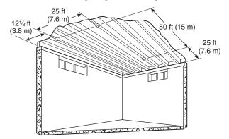
In addition to the special requirements for heat detectors installed on ceilings with exposed joists, reduced spacing also might be required due to other structural characteristics of the protected area, possible drafts, or other conditions that could affect detector operation.
