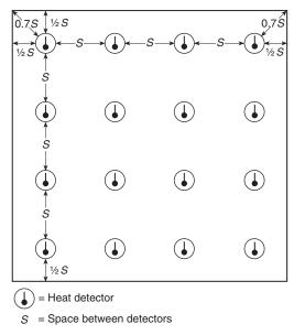
Figure A-2-2.4.1(b) Line-type detectors — spacing layouts, smooth ceiling.
