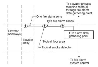
Figure A-3-9.3.7(b) Elevator zone — elevator installed after fire alarm system.
