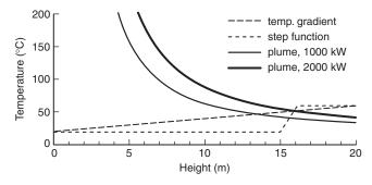
**B-4.1.2.3.8.4** Step Function Temperature Gradient Spaces. If the interior air temperature exhibits a discrete change at some elevation above the floor, the potential for stratification can be assessed by applying the plume centerline temperature correlation. If the plume centerline temperature is equal to the ambient temperature, the plume is no longer buoyant, loses its upward momentum, and stratifies at that
