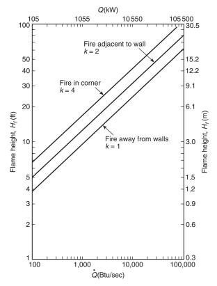
**B-2.3.2.1.3 Example.** What is the average flame height of a fire with a heat release rate of 1000 Btu/sec located in the middle of a compartment?
