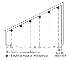
Figure A-2-2.4.5.1 Detector spacing layout, solid joist construction.
