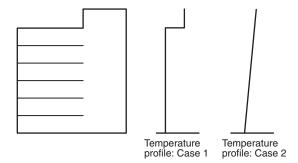
Figure B-4.1.2.3.8.3(b) Indoor air and plume temperature profiles with potential for intermediate stratification.
