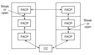
Style 7 fiber network where the panel has a two-way path communications capability with the two breaks now breaking into two LANs, both functioning as independent networks with the same Style 7 capabilities.
