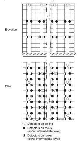
Figure A-2-3.6.5(a) Detector location for solid storage (closed rack) in which transverse and longitudinal flue spaces are irregular or nonexistent, as for slatted or solid shelved storage. Figure A-2-3.6.5(b) Detector location for palletized storage (open rack) or no shelved storage in which regular transverse and longitudinal flue spaces are maintained.
