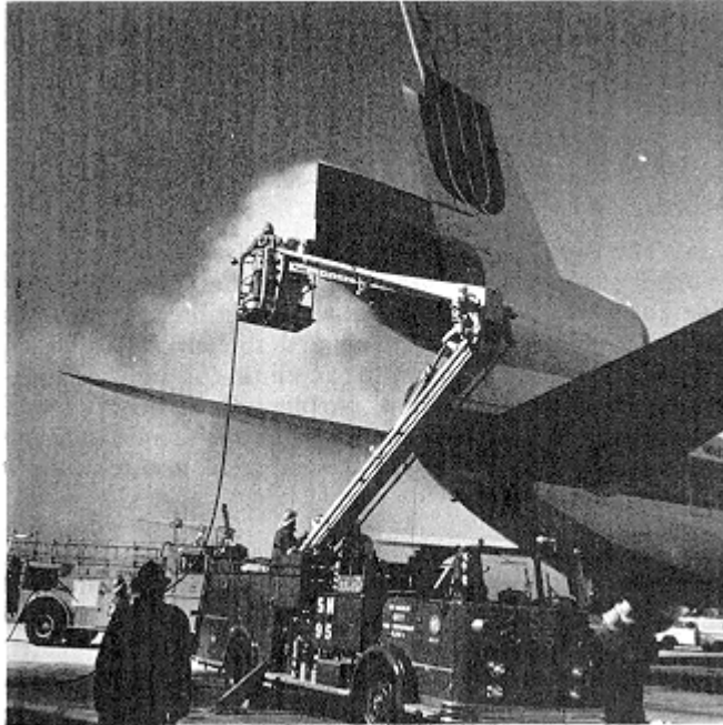
Figure B-2 Elevated platform vehicle.
