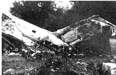
Figure 12-1(b) The nose of the DC-9 sheared off on impact with trees and skidded down a residential street.
