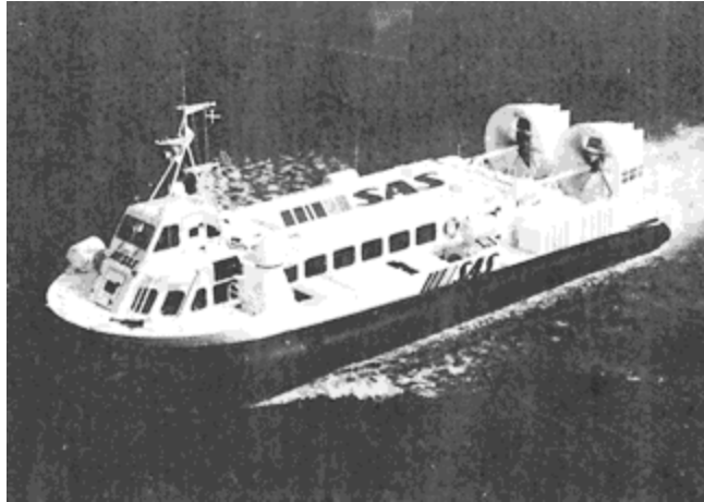
Figure A-3-16 The “Winchester” Class Hovercraft (built by the British Hovercraft Corporation), which is in service at the Auckland International Airport in New Zealand. It is utilized to protect aircraft operations that are largely over the Manukau Harbor that borders the airport. The primary mission is rescue of occupants in the event of an accident in the harbor or mudflats (which exist at low tide).
