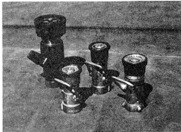
Figure 12-7 Photo shows a variety of typical spray nozzles currently used by structural fire departments. All have the feature of adjustable spray patterns and straight stream settings. Some also have variable flow settings. Most fire chiefs agree that a nozzle setting of 30 degrees provides the best pattern for fighting flammable liquid fires with either water, AFFF, or FFFP solutions.
