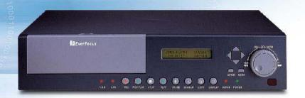
The EDSR100 single channel digital video recorder is the first true VCR replacement designed particularly for the security industry, seamlessly combining high-resolution video multiplexing and digital recording. The EDSR100 can record at speeds up to 60/50 images per second with NTSC/PAL formats and
