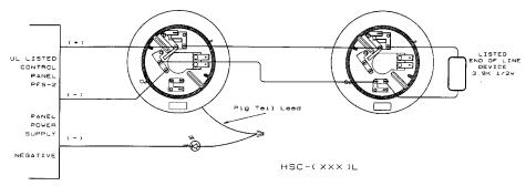
Nominal alarm current shown at 24V. Polarized with annunciator output.
