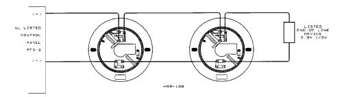
Non polarized, not current limited. No annunciator output.
