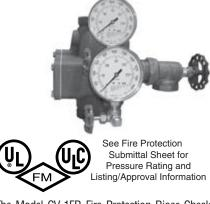
The Model CV-1FR Fire Protection Riser Check Valve is a compact and rugged swing-type unit that allows water flow in one direction and prevents flow in the opposite direction. A resilient elastomer seal facing on the spring loaded clapper ensures a leak tight seal and non-sticking operation. All Model CV-1FR Riser Check Valves are designed to minimize water hammer caused by flow reversal.
