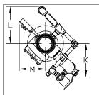
Model J-1 Alarm Check Valve Vertical Trim, and Pressure Switches Must be Ordered Separately Refer to Technical Data.
