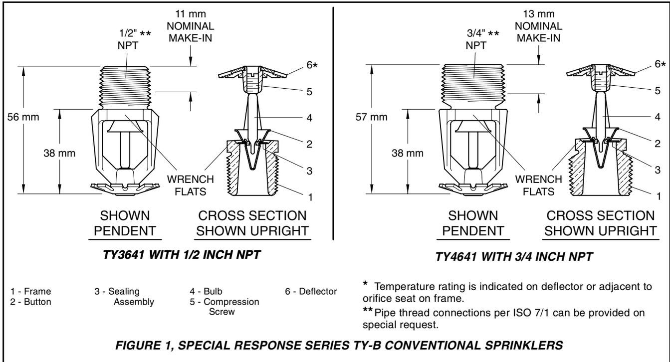
to 27 Nm. A maximum of 40 Nm of torque is to be used to install sprinklers with 3/4 NPT connections. Higher levels of torque may distort the sprinkler inlet and cause leakage or impairment of the sprinkler.
